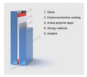
In a normal (OFF) position the electrochromic layer is transparent (unlike some other technologies). When 2-V voltage is applied (ON-position), within seconds the glass becomes tinted in a preset shade of blue colour:
